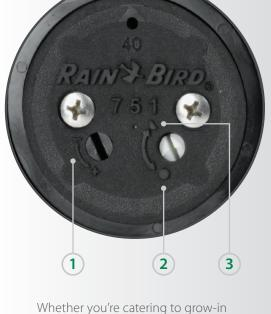
or just trying to get more from a limited water supply, Rapid-Adjust Technology lets your staff make easy arc adjustments with the turn of a screw. MemoryArc retains two part-circle arc settings, so you can shift between full- and part-circle operation in seconds.
